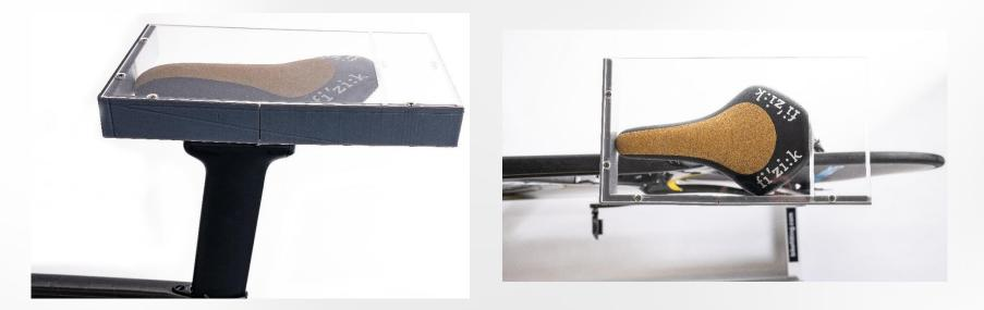
Step 8: Place the extension target (F) near the end of the extension closest to the laser tool (C) and secure it in place using the thumb screw.
