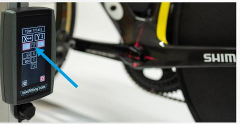
Step 10a: Measure the saddle position by aligning the crosshair laser with the engraved crosshair on the saddle target and pressing the "S" button on the screen. If the saddle position is compliant, the button will turn green, if it is not compliant, it will turn red.
