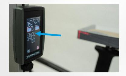
Step 10b: Measure the saddle tilt by visually checking the horizontal laser line. If the laser line falls between the 9deg engraved lines on the saddle target, the saddle tilt is compliant. If the horizontal laser line falls outside of the two engraved lines, the saddle tilt is not compliant. The tilt can also be measured by placing the digital protractor on the top of the saddle target.
