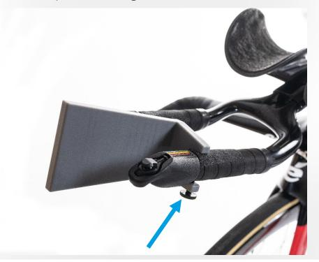
Step 9: Set the bottom bracket of the bicycle as the reference point for the measurements by aligning the crosshair laser with the bottom bracket and pressing the "ZERO BB" button on the screen
