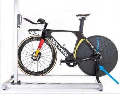
Step 7: Place the saddle target (E) on the saddle, ensuring the nose of the saddle is flush with the front wall of the pointer and that the engraved wall is perpendicular to the laser tool (C).
